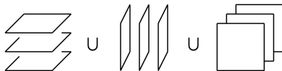
Figure 5: The multidirectional multislice decomposition of a digital point set in a three-dimensional digital space.
