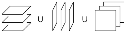
Figure 4: The multidirectional multislice decomposition of a digital point set in a three-dimensional digital space.
